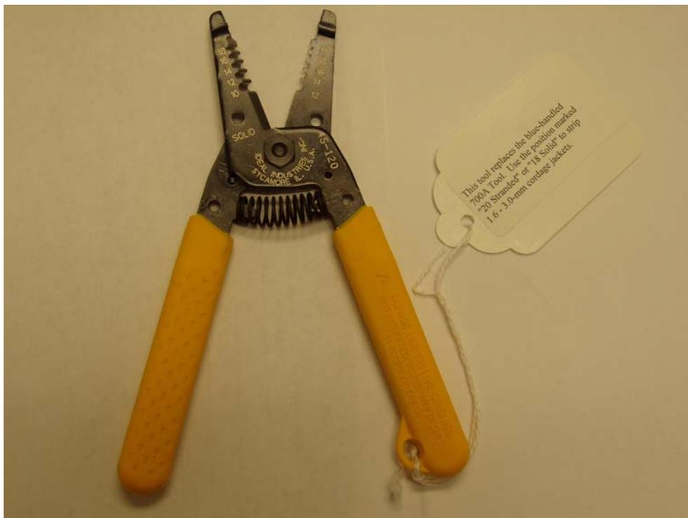
Figure 2. Ideal 45-120 Strip Tool w/ Note Card Attached
