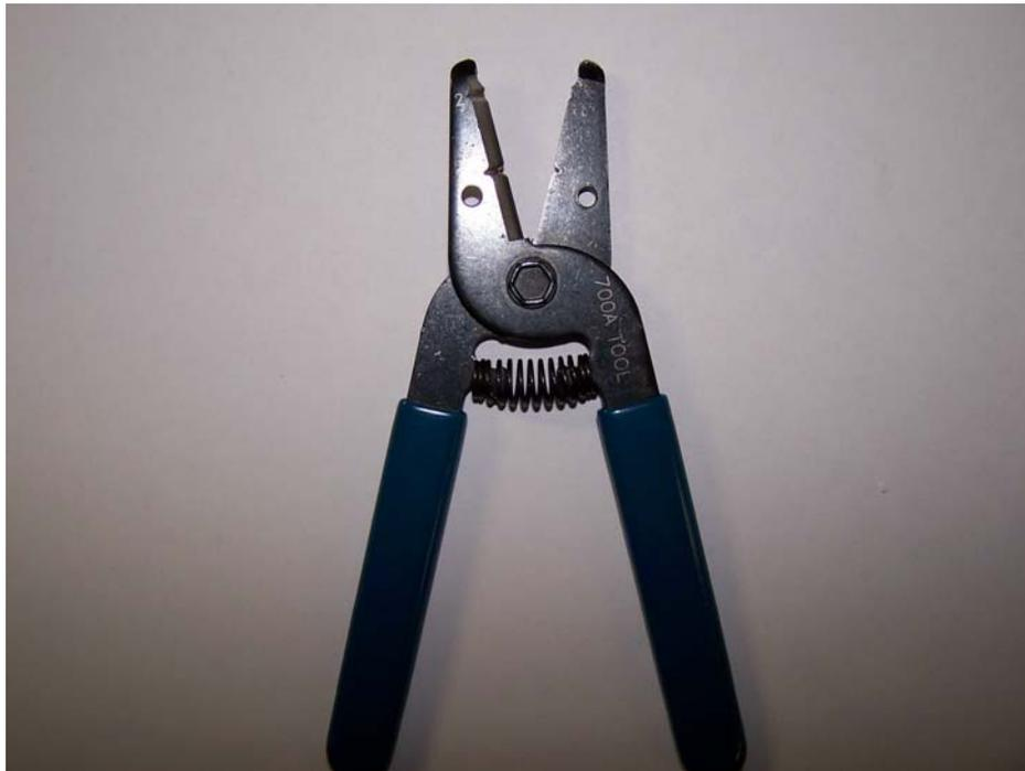
Figure 1. Blue-Handled 700A Stripping Tool
